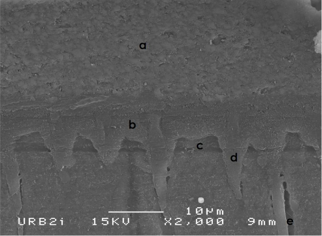
Key: a: Reflectys composite; b: Iperbond Ultra adhesive; c: hybrid layer (penetration of adhesive into the intertubular dentine); d: resinous cord (penetration of adhesive into the tubule); e: dentinal tubule
