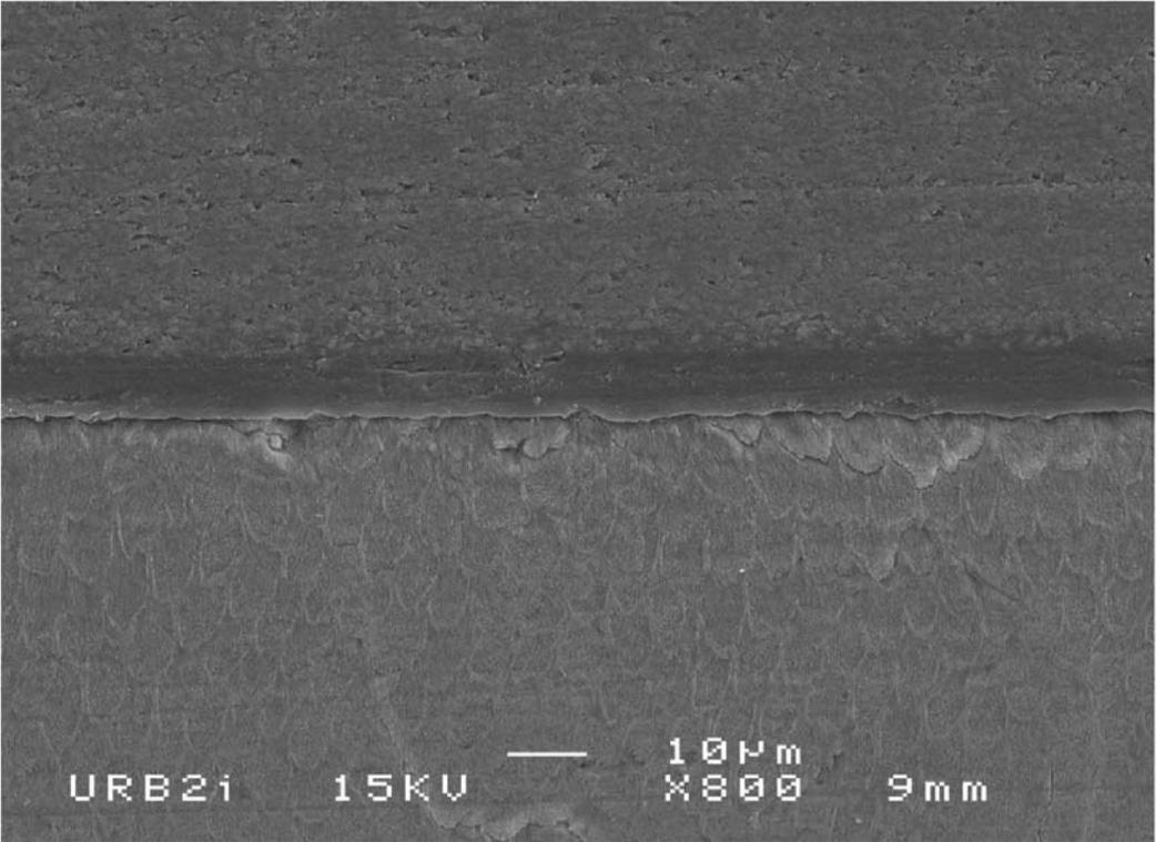
Fig. 4: Group 2: Reflectys/enamel interface cemented using Iperbond Ultra without preliminary etching (x2000)
