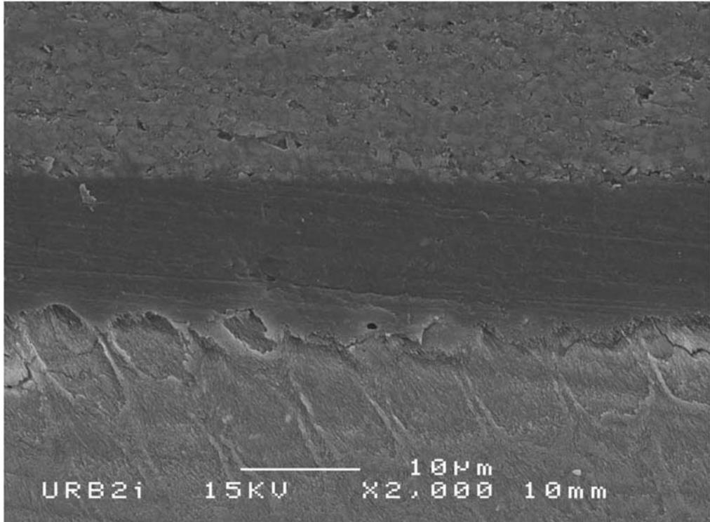
Fig. 3: Group 2: Reflectys/enamel interface cemented using Iperbond Ultra without preliminary etching (x800)
