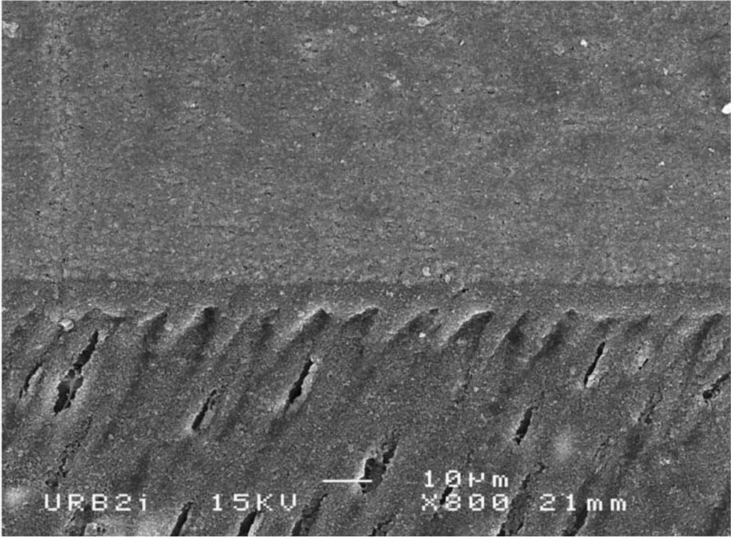
Fig. 6: Group 3: Reflectys/dentine interface cemented using Iperbond Ultra with preliminary etching (x2000)
